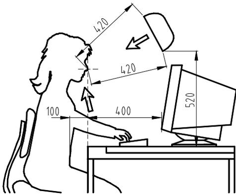
Fig. 7. Details of the positioning of the Round Movable Panel and the Vertical Desk Grille.
