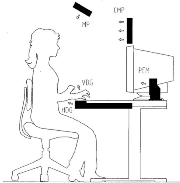
Fig. 1. Personalized ventilation. Examples of tested air supply terminal devices (ATD): Movable Panel (MP), Computer Monitor Panel (CMP), Vertical Desk Grill (VDG), Horizontal Desk Grill (HDG), and Personal Environments® Module (PEM).
