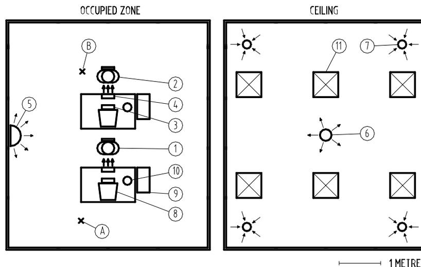
Fig. 6. Office plan: (1) front thermal manikin – 23 sections, (2) back thermal manikin – 16 sections, (3) Personalized ventilation – RMP, (4) Personalized ventilation – VDG, (5) Displacement ventilation supply, (6) Mixing ventilation supply, (7) Exhaust, (8) 17" computer monitor – 70 W, (9) Computer tower – 75 W, (10) Desk lamp – 55 W, (11) Ceiling light fixture – 6 W, (A)-(B) Measurement positions.
